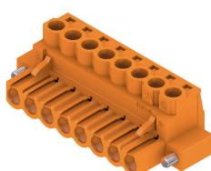
Female plug with clamping-yoke screw system for connecting wires with straight (180°) outlet direction. The female connectors provide space for labelling and can be coded. Fastened by means of a flange or release latch. The also provide an integrated plus/minus screw, protection against faulty insertion of the wire, and they are delivered with open clamping yokes. HC = High Current.
