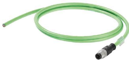
Assembled IE cables, PROFINET, Cat. 5, PUR, green, drag-chain compatible, M12
