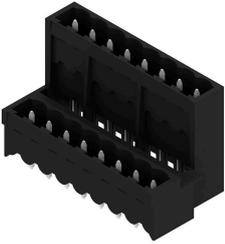
High-temperature resistant, double level, laterally offset, closed ended male header, with solder flange option. 1.5 mm solder pin suitable for reflow soldering. 3.2 mm solder pin suitable for reflow and wave soldering. The pin headers provide space for labelling and can be coded.
