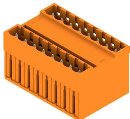
2-tier male header with parallel pin arrangement. The solder pin length is optimised for wave flow soldering. The pin headers provide space for labelling and can be coded.
