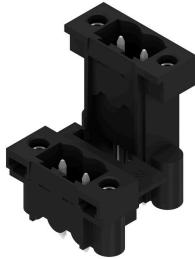
High-temperature resistant, double level, laterally offset, closed ended male header, with solder flange option. 1.5 mm solder pin suitable for reflow soldering. 3.2 mm solder pin suitable for reflow and wave soldering. The pin headers provide space for labelling and can be coded.
