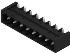
High-temperature-resistant, straight, open pin header. Packed in box or tape. On tape and with 1.5 mm solder pin, optimised for automatic assembly. 3.2 mm solder pin suitable for reflow and wave soldering. The pin headers provide space for labelling and can be coded. HC = High Current.
