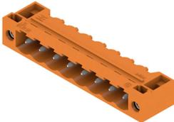
Pin headers made from glass-fibre-reinforced plastic with 90° wire outlet; optimised for wave soldering. The flange variant (F) can be screwed onto the respective counter piece or the circuit board. There is no need for an extra screw to connect the circuit board when the solder flange (LF) version is used. This also protects the solder points from mechanical strain. All pin headers can be manually coded or ordered pre-coded. HC = High Current.
