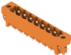
Pin headers in glass-fibre-reinforced plastic with straight wire outlet; optimised for wave soldering. The flange variant (F) can be screwed onto the respective counter piece or the circuit board. There is no need for an extra screw to connect the circuit board when the solder flange (LF) version is used. This also protects the solder points from mechanical strain. All pin headers can be manually coded or ordered pre-coded. HC = High Current.
