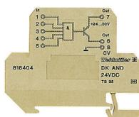
Logic functions AND, NAND, OR and NOR in modular terminal format with a rated cross-section of 4 mm<sup>2</sup>. They each have five inputs which are fed – with logic gating – via a 24 V/20 mA PNP output. The logic components can be used for many applications involving the coupling of digital sensor/actuator signals with automation devices.
