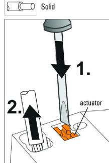
Push the actuator with a screwdriver to remove the wire.
