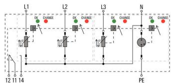
Schematic circuit diagram
