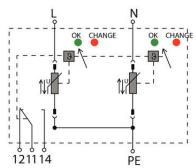
Schematic circuit diagram
