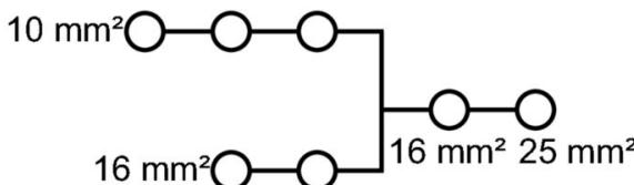
Conductor connection data according to IEC 60947-7-1 (Cu)
