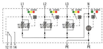
Schematic circuit diagram
