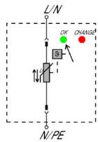
Schematic circuit diagram
