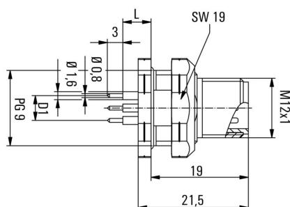
L (board-to-board distance) = 5.5mm D1 = 5,0 mm
