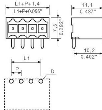
$L1 = 31.50 \text{ mm} | P = 3.50 \text{ mm}$
