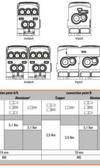
Conductor connection data according to UL 1059 (Al+Cu)
