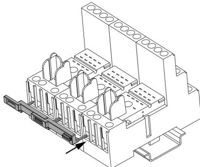
Plug the cross connection into wire-connection opening
