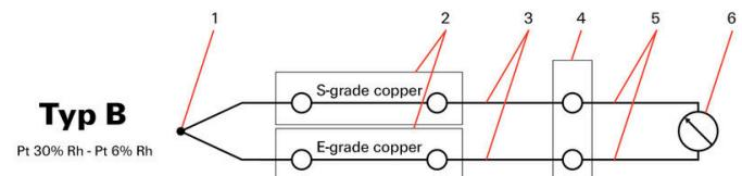
1. Thermocouple (sensor)
