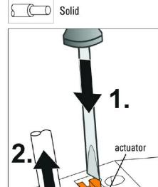
Push the actuator with a screwdriver to remove the wire.
