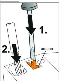
Stranded wires without ferrule can be inserted by pushing down the actuator using a screwdriver.
