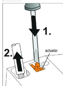
Push the actuator with a screwdriver to remove the wire.
