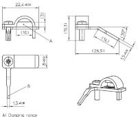
A) Clamping range B) Contact pin for cross sections 1,5mm² Units are in millimeters (mm) and degrees (°)
