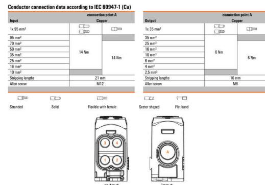
Conductor connection data according to 1059 (Al+Cu)
