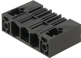
Single-row, high-current male header, for side-by-side mounting without sacrificing any poles, or with patented flange for fast locking without tools. Maximum connection and operating reliability thanks to a mating profile that prevents incorrect connection, with unique coding diversity and additional fastening in the flange. 3.5 mm pin length is optimised for wave soldering, plug-in direction 90° to solder pins.
