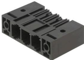
Single-row, high-performance male header for side-by-side mounting without sacrificing any poles or with patented flange for fast fixing without tools. Maximum connection and operating reliability thanks to a mating profile that prevents incorrect connection, with unique coding diversity and additional fastening in the flange. 3.5 mm pin length is optimised for wave soldering, plug-in direction 270° to solder pins.
