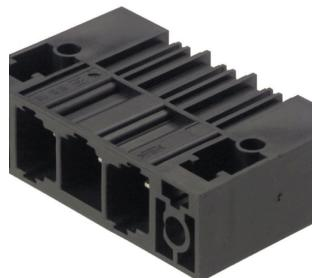
Single-row, high-current male header, for side-by-side mounting without sacrificing any poles, or with patented flange for fast locking without tools. Maximum connection and operating reliability thanks to a mating profile that prevents incorrect connection, with unique coding diversity and additional fastening in the flange. 3.5 mm pin length is optimised for wave soldering, plug-in direction 90° to solder pins.
