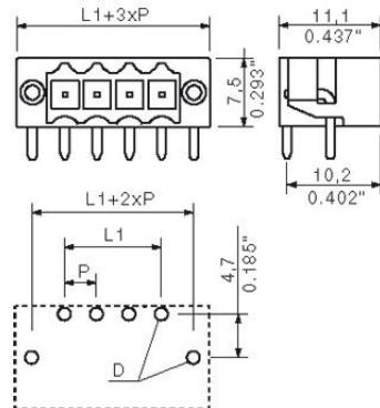
$L1 = 66.50 \text{ mm} | P = 3.50 \text{ mm}$
