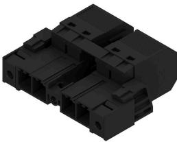
180° inverted male header with PUSH IN connection technology for field wiring in 6 mm<sup>2</sup> with 7.62 pitch as "three-flange variant" for housing passage. Suitable for housings with a max. wall thickness of 2 mm.
