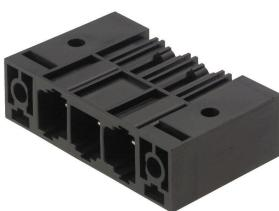
Single-row, high-performance male header for side-by-side mounting without sacrificing any poles or with patented flange for fast fixing without tools. Maximum connection and operating reliability thanks to a mating profile that prevents incorrect connection, with unique coding diversity and additional fastening in the flange. 3.5 mm pin length is optimised for wave soldering, plug-in direction 270° to solder pins.
