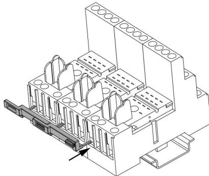
Plug the cross connection into wire-connection opening
